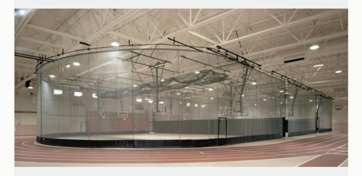
The Radius Dividing Curtain system is custom engineered for individual facilities, and is designed to allow a wrap around curtain to enclose a court.
